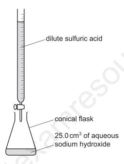
25.0 cm<sup>3</sup> of aqueous sodium hydroxide of concentration 0.100 mol/dm<sup>3</sup> was neutralised by 25.0 cm<sup>3</sup> of dilute sulfuric acid of concentration 0.0500 mol/dm<sup>3</sup>. The equation for the reaction is shown. This is **reaction 1**.
