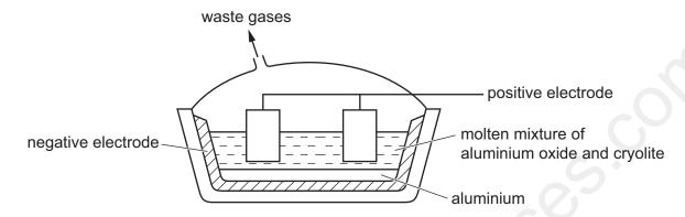
(i) Give **two** reasons why the electrolysis is done using a molten mixture of aluminium oxide and cryolite instead of molten aluminium oxide only.
