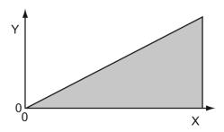
The shaded area represents the total strain energy stored in stretching the wire.
