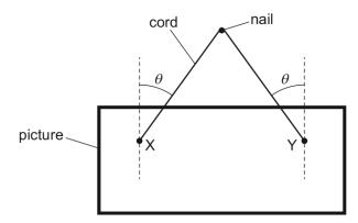
The tension in the cord is T. The angle between the cord and the vertical is  $\theta$  on both sides.
