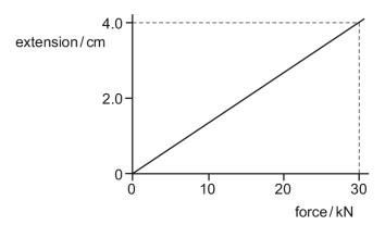
What is the strain energy in the spring when the extension is 4.0 cm?
