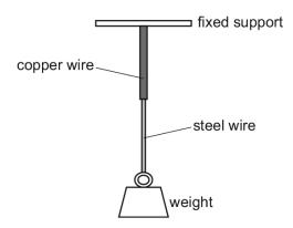
The combination wire is stretched by a weight added to its end. Both the copper and the steel wires obey Hooke's law.
