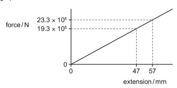
What is the increase in strain energy in the cable when the lorry is crossing the bridge?
