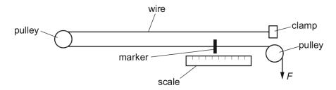
The wire passes from a clamp, around a frictionless pulley, and then to a second frictionless pulley where loads F are applied to it. A marker is attached to the wire so that the total length of wire between the clamp and the marker is initially  $3.70 \, \text{m}$ . A scale is fixed near to this marker.
