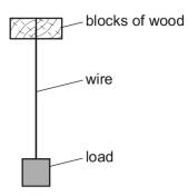
A second wire is made of the same material, but of diameter 2*D* and length 3*L*. Both wires obey Hooke's law.
