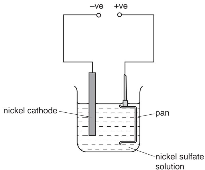
Which change is necessary to plate the pan with nickel?
