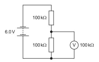
A voltmeter of resistance  $100 \, k\Omega$  is connected across one of the resistors.
