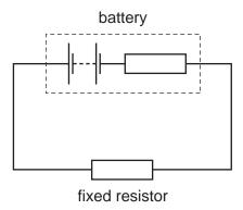
The battery is replaced by one of the same e.m.f. but with a larger internal resistance.
