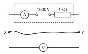
A connecting lead of negligible resistance is connected between points X and Y.
