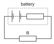
When 100 C flows around the circuit, 120 J of electrical energy is dissipated in resistor R and 20 J in the battery's internal resistance.
