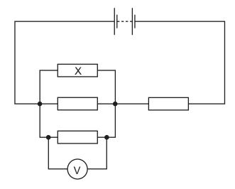
The voltmeter reads 6.0 V. The battery has negligible internal resistance.
