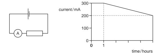
How much charge passes through the cell during this time?
