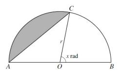
The diagram shows a semicircle ACB with centre O and radius r. The angle BOC is x radians. The area of the shaded segment is a quarter of the area of the semicircle.
