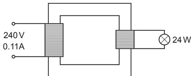
The input current to the transformer is 0.11 A and the input voltage is 240 V. The useful output power of the transformer is 24 W.
