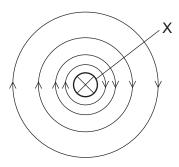
The arrows on the field lines show the direction of the force on
