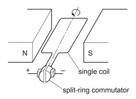
The split-ring commutator reverses the current in the coil as the coil rotates.
