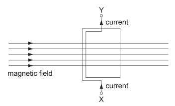
In which direction does the coil move?
