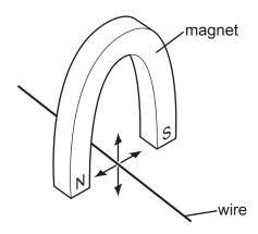
The current in the wire can be reversed. The poles of the magnet can also be changed over.
