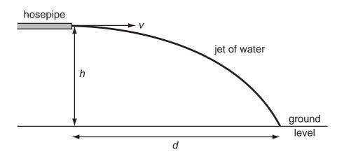
The jet of water emerges with a horizontal velocity v. The hosepipe is fixed at a height h above the ground. The water jet hits the floor at a horizontal distance d from the nozzle tip. The gravitational field strength is g.
